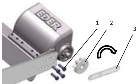
Fig. 2: Fastening the peeling head to the support
