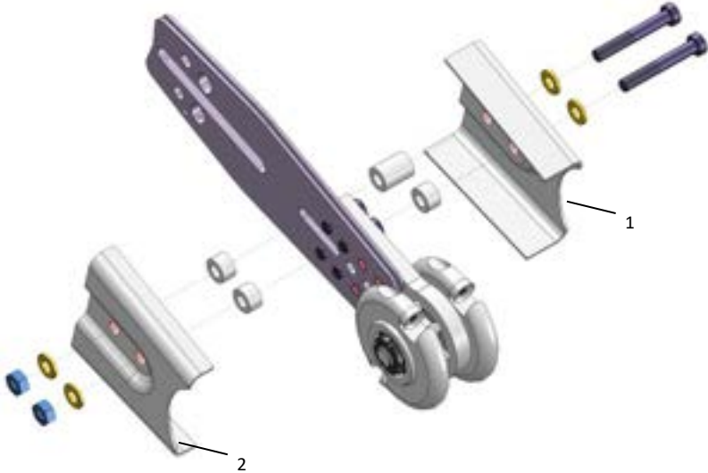
Fig. 8. Mounting the protective plates
